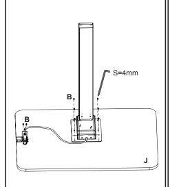
Install the base support bracket (N) to the top of the base (M) with x4 M6x14 bolts (H), and press the plastic bushings (I) into the openings in the base and base support bracket. Assemble the base to the leg (L) using M6x16 bolts (C), then tighten all bolts with the Allen wrench (D).
